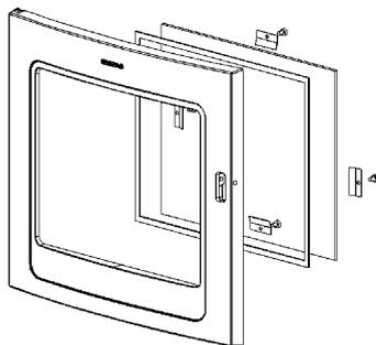
1. When you open the door, you will find two small M4 unbraco screws, one in each hinge. Unscrew the two screws, lift the door off the hinges and place it face down on a sheet of cardboard or other nonabrasive fabric.
