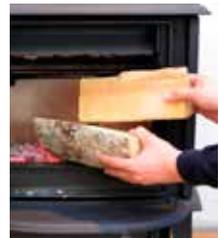
When refuelling your stove, it is recommended that you open the stove door gently for the first 2 - 3 centimetres, then wait for a few seconds for the pressure in the flue to equalise; you are now safe to proceed and open it all the way. By using this technique smoke spillage can be eliminated particularly in poor chimney draft conditions. The stove door should not be opened when the stove is being fired vigorously.
