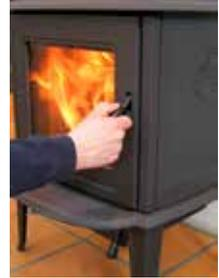
9. Once the new fuel has taken, adjust the secondary air amount to the desired setting; optimal combustion will continue until glowing embers are produced. Under normal chimney draft conditions, expect to refuel your stove every 60 - 70 minutes.
