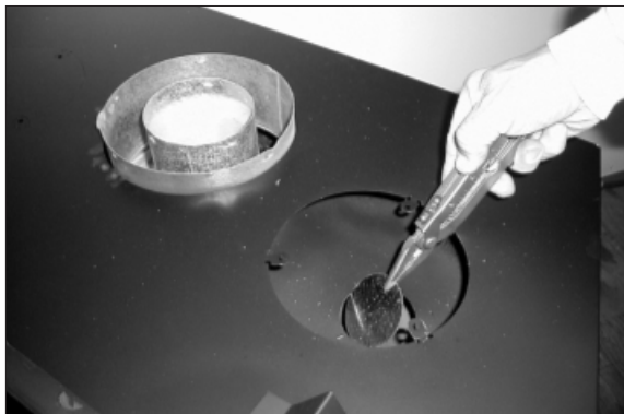
Figure 4.3, Second Knock-out Removal
