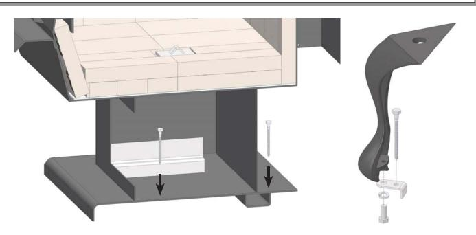
In mobile home installations, the stove must be securely fastened to the floor using the tie-downs provided in the Outside Air kit. (For the pedestal model, remove the ash drawer to access the screw down holes. For the Leg model, use the Leg Anchor Kit (P/N ZR8039) to secure stove to floor.) ALSO, a #8 ground wire must be attached to the stove and an appropriate ground.
