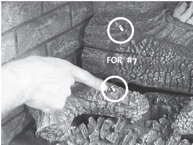
Figure 47. #7 Log: Engage the underside holes with the pins in Log #1 and Log #2.
