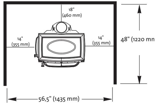
Side Loading Door must be locked in alcove installations.
