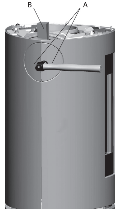
Figure 10. Removing the rear exit outlet knock-outs.
