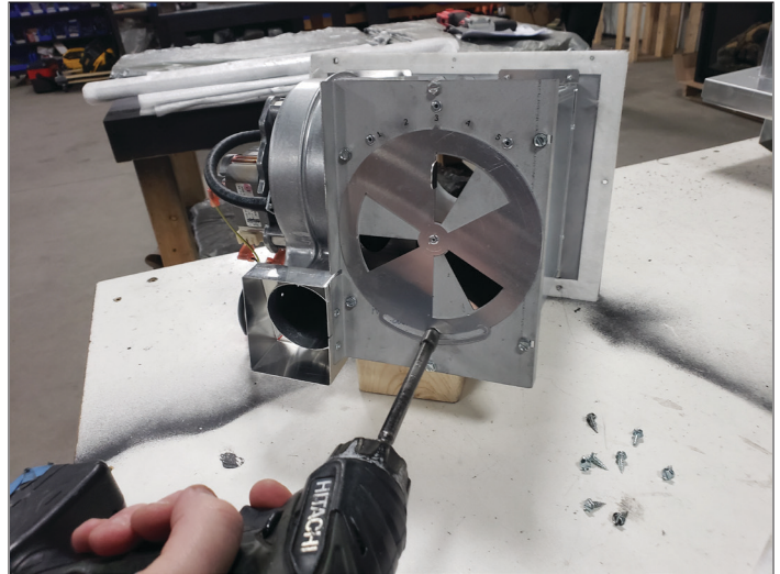
Figure 2.8, Loosen Locking Screw
