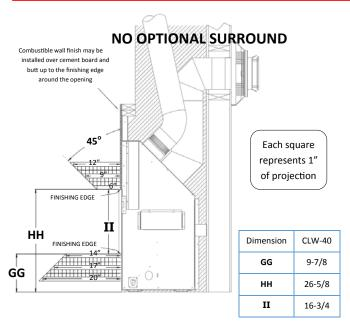
Below shows where to end masonry finishing materials, when measuring from the finishing edge. This allows the installation of an Optional Surround. This is important, due to the fact that most masonry finishing materials will not fit behind the optional surround if one is installed.
