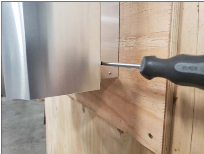
Figure 2.4, Remove Cover Assembly
