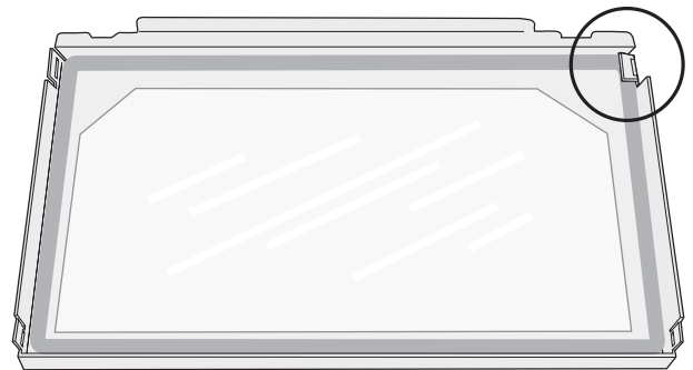
Figure 74. Bend the retainer tabs back enough to release the glass panel.
