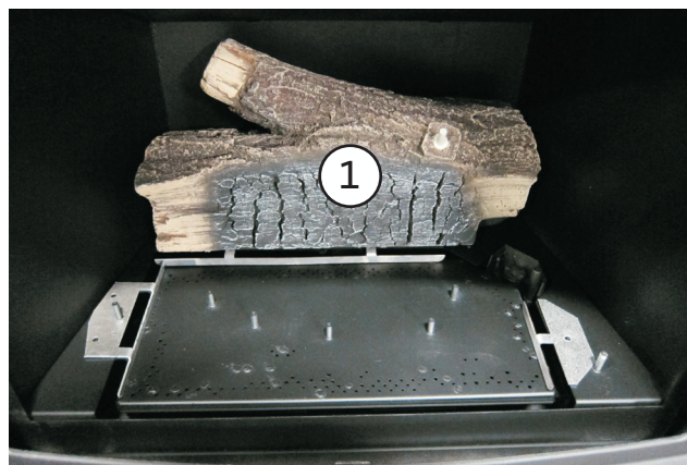
Figure 30. Locate the Rear Log over the two pins on the back shelf of the burner skirt.
