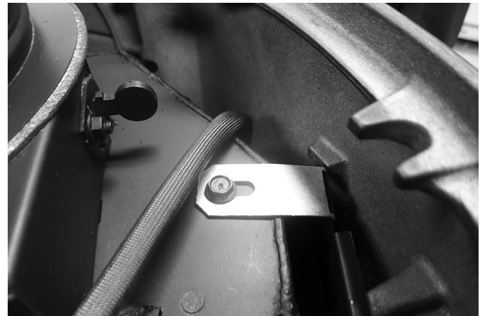
Figure 16.2. Remove the firebox-to-side plate bolt.
