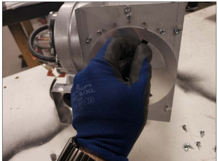
Figure 2.7, Adjust the Draft Bypass
