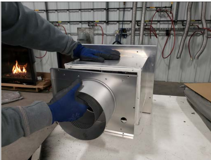
Figure 3.7, Removing Exhaust Assembly
