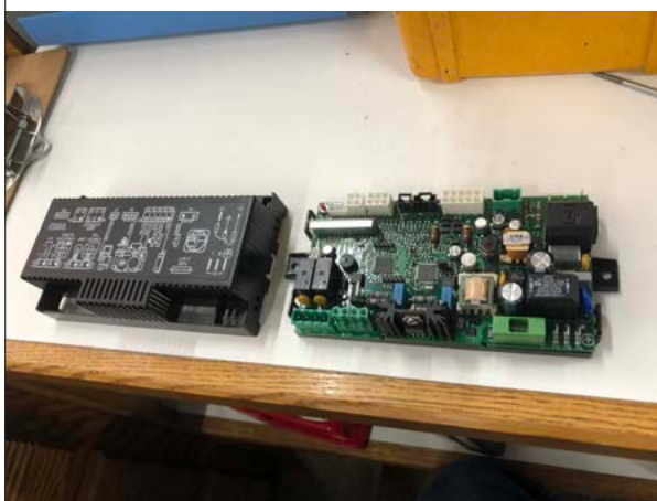
Figure 4.1, Remove Control Board Cover
