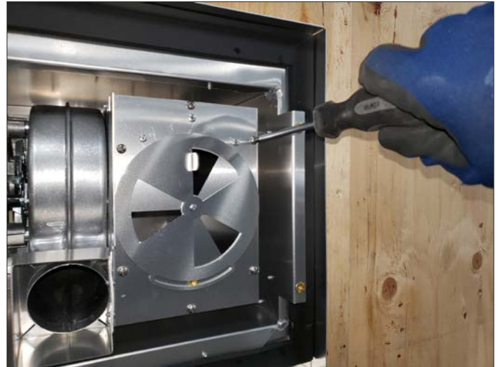
Figure 5.2, Exhaust Assembly Screws
