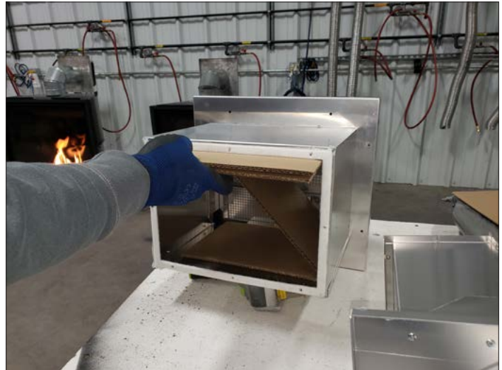
Figure 3.9, Remove Corrugated Shipping Pads
