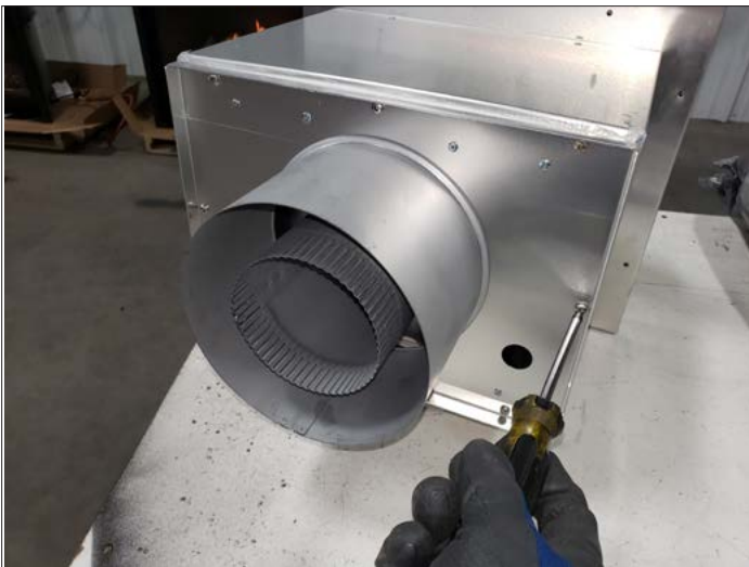
Figure 3.6, Remove Back Assembly
