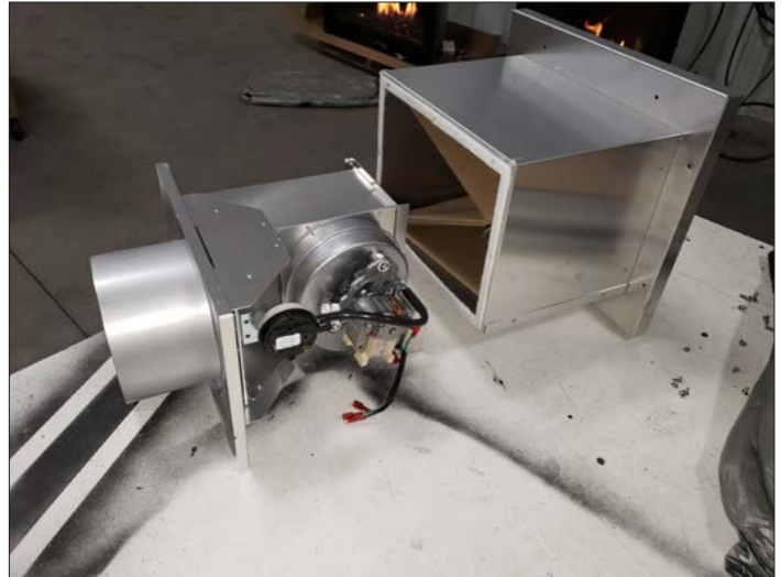
Figure 3.8, Exhaust Assembly Removed
