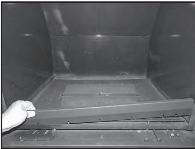
Figure 89: Inserting front trim piece.
