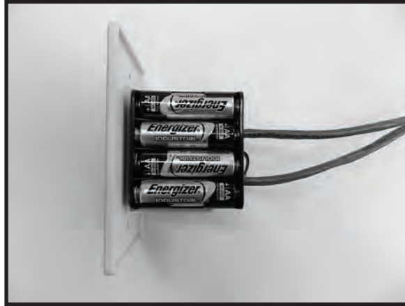
Figure 34: Wall switch - battery side.
