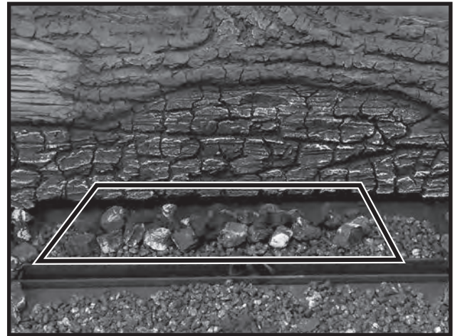
Figure 78: Large ember chunks on rear burner.
