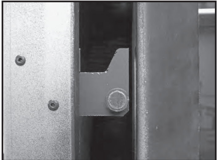
Figure 97: Upper hook for safety screen.
