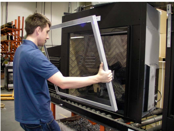
Figure 16b. Lift screen off retainer slides.
