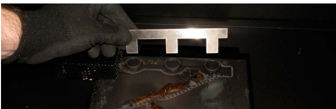
Figure 23.c Pushing the Rock Guard down into place.
