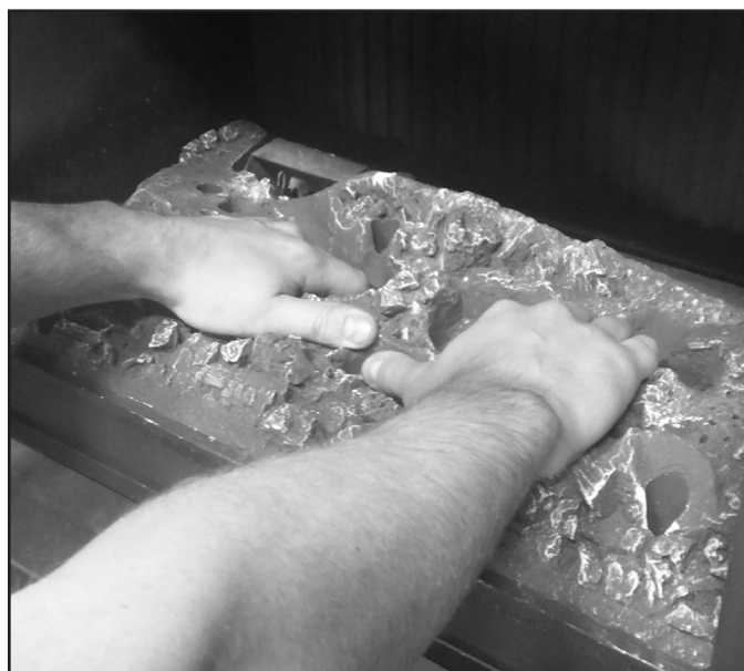
Figure 22. Burner Removal - Correct Hand Placement
