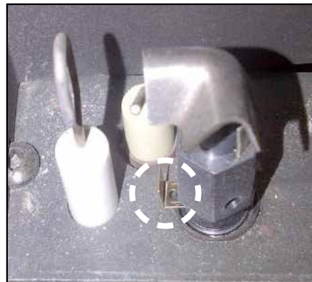
Figure 24. Pilot Slider set to LP
