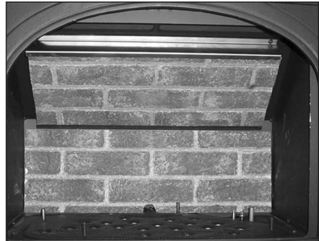
Figure 64: Back brick panel in place.
