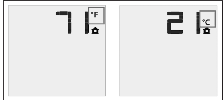
Figure 7: Remote Control Display in Farenheit and Celcius.
