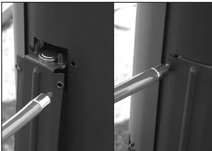
Figure 55: Spill switch installation.
