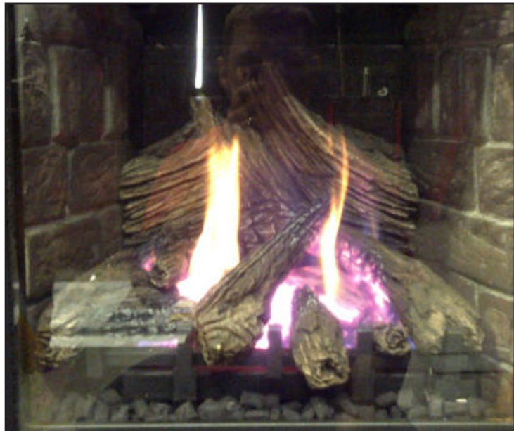
Figure 47. Complete log set-up with coal nuggets burning.
