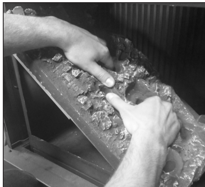
Figure 26. Burner Removal - Rotate 45 degrees
