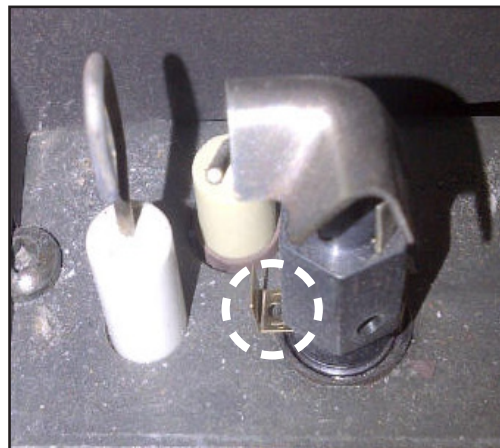
Figure 27. Pilot Slider set to LP
