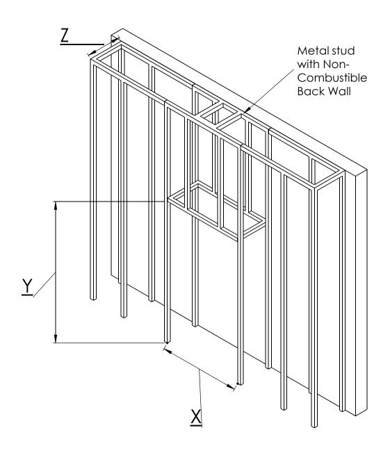
NOTE: Dimension 'Y' uses legs at default lowest height 4" below the unit with glass beginning 10" above the floor. Increase leg height and Y dimension for higher viewing window.
