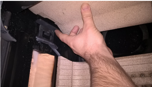
Remove the steel skamol bracket, holding the Upper baffle plate.
