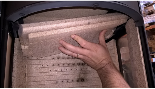
Remove the Back left skamol corner, by carefully lifting it up and out.
