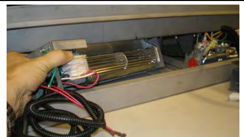
3. Insert fan and place at right rear corner of unit. See Component Locations Section in manual.
