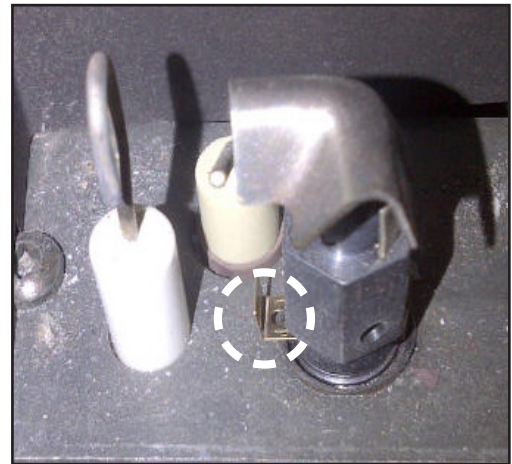
Figure 22. Pilot Slider set to LP
