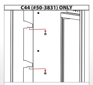
Use the fasteners in the side of the cabinet to attach the surround.
