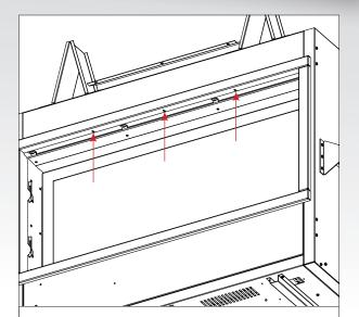
6) If surround starts to warp after usage, use self-tapping metal screws (not included) in the slots located on the underside of the top surround piece. (screen removal required, see steps 2 and 5)
