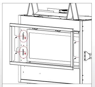
4) For C34, C60, and C72 models insert the notched tabs on the surround into the forward most slots in the stove (circled above).
