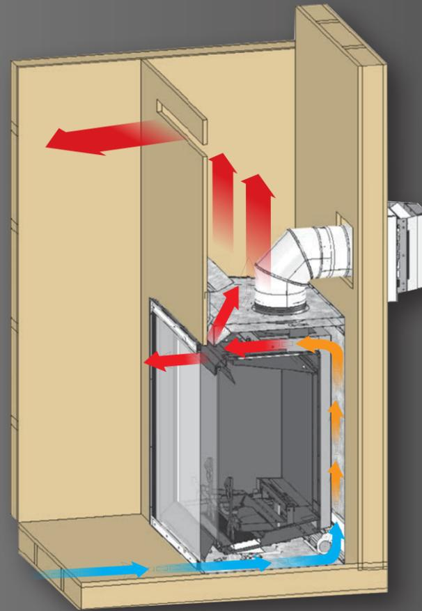
*Convective heat that rises from the fireplace is captured in the chase and channeled through the vent using the Cool Surface System.*
