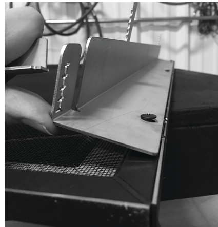
Figure 4.10, Screw Location on Hanging Bracket
