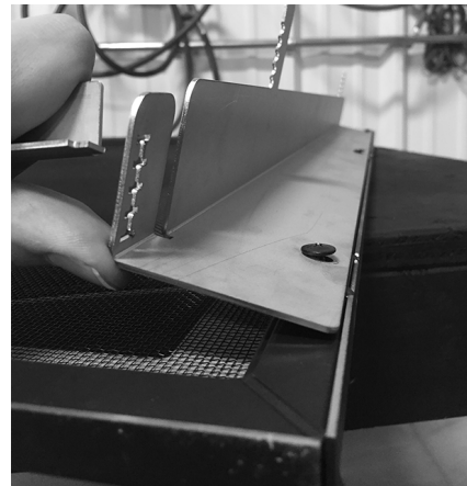
Figure 4.10, Screw Location on Hanging Bracket
