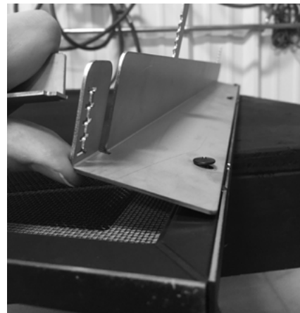
Figure 4.10, Screw Location on Hanging Bracket
