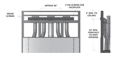
Insert Brace to secure unit to stud frame
