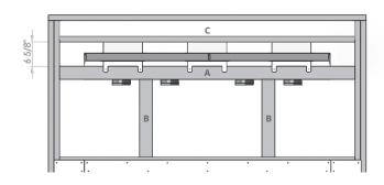
The opening should be a minimum of 33" from the top of the fireplace and a minimum of 3" from the ceiling.
