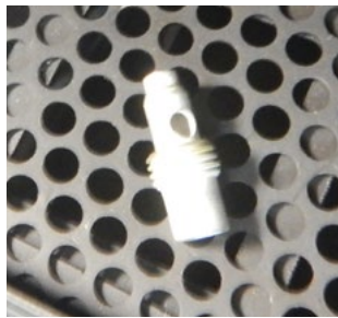
Figure 13.e Removing the pilot hood, orifice
