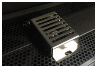
Figure 13. Removal of pilot cover
