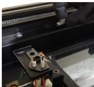
Figure 13.f Insert propane orifice, reassemble burner
