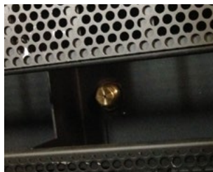
Figure 13.c Removing the orifice
