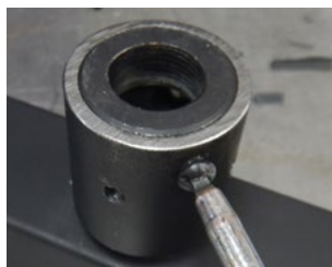
Figure 13.c Removing the orifice
