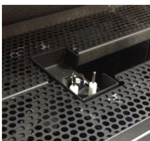
Figure 13.e Removing the pilot hood, orifice
