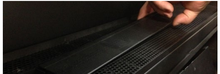
Figure 13.b Loosening the venturi
