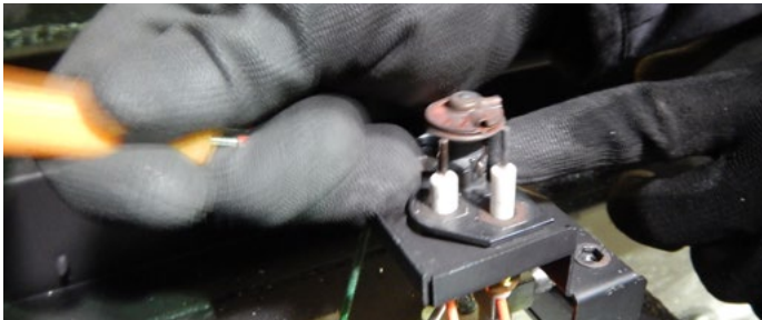
Figure 13.d Removing the spring clip
