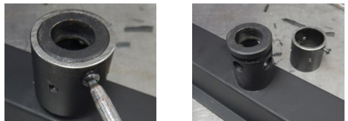
Figure 13.c Removing the orifice
