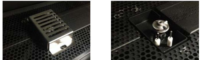
Figure 13. Removal of pilot cover
