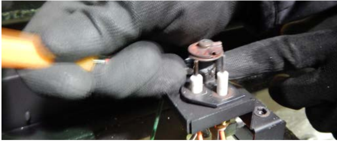
Figure 13.d Removing the spring clip
