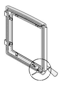
2. Turn the handle counter clock wise one turn to increase pressure. To reduce the pressure, when installing a new gasket for example, turn clock wise.
