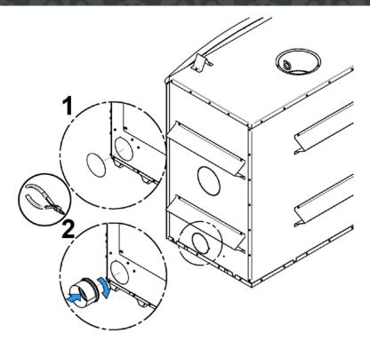
3. Flip the fireplace lower decorative louver. Install the blocking plate **(F)** included with the fireplace, on the front opening of the air control housing. Using a screwdriver, secure with four screws located in the user's manual. Installing the block off plate will redirect air supply directly to the firebox instead of the area under the unit for combustion.
