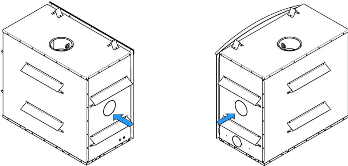
This kit allows distributing heat to another room up to 50 feet (15 m) of the fireplace. The insulated flexible pipe (not included in the kit) must be HVAC type pipe and must comply with ULC S110 and/or UL 181, Class 0 or Class 1 Standards and must withstand temperatures up to 250 °F.
