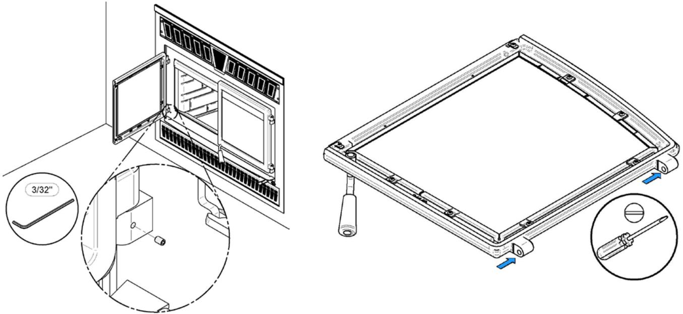
Using a flat screwdriver, turn the adjustable hinge rods in the direction shown to adjust the doors. Tighten all door hinge pressure screws when they are at the desired positions.
