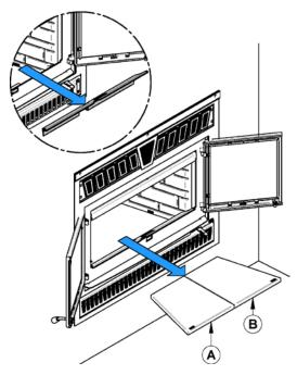
3- Remove the rear refractory slab (E).
