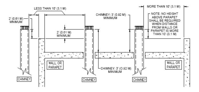
For installations where more than one chimney is located in the same non-chase or within the same area, we suggest that their terminations be separated by at least 16" (410 mm) horizontally, and 18" (460 mm) vertically. This separation is to prevent smoke migrating from one chimney to another.
