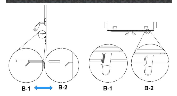
In the B position, it is also possible to close the air supply manually if a power failure occurs by pushing the small lever to the left.
