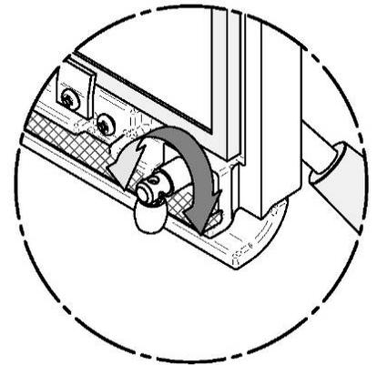
3. Re-install the split pin with a small hammer.
