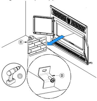
To install new refractory slabs, follow the above steps in reverse.
