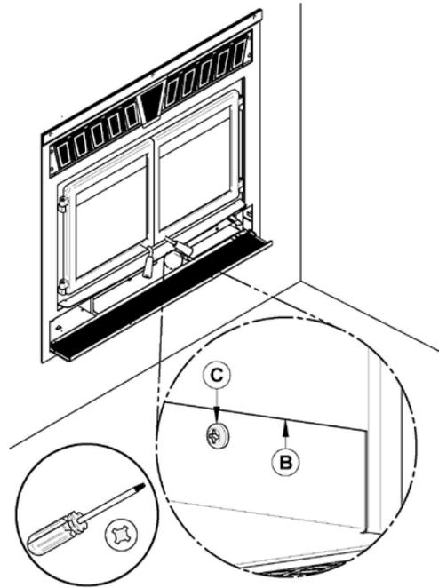
3. Remove and keep the heat shield (B) and the 4 screws (C).
