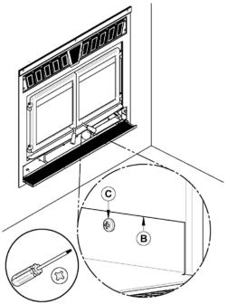
3. Remove and keep the heat shield **(B)** and the 4. Cut the Tie wrap **(D)**. 4 screws **(C)**.
