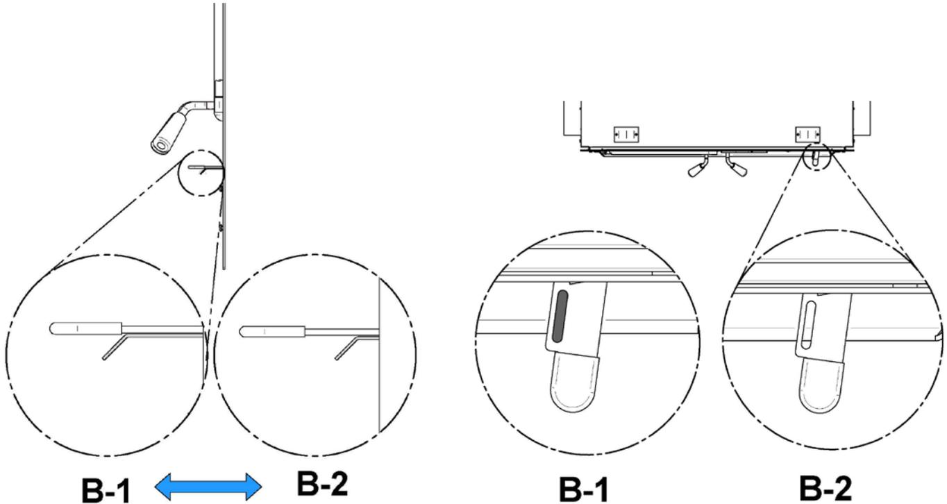
In the B position, it is also possible to close the air supply manually if a power failure occurs by pushing the small lever to the left.
