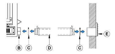
\*For a pipe length less than 20 ft, use a 5" pipe diameter. For a pipe length of more than 20ft, or having more than two deviations, use a 6" pipe diameter. The maximum pipe length is 30 ft (9 m).
