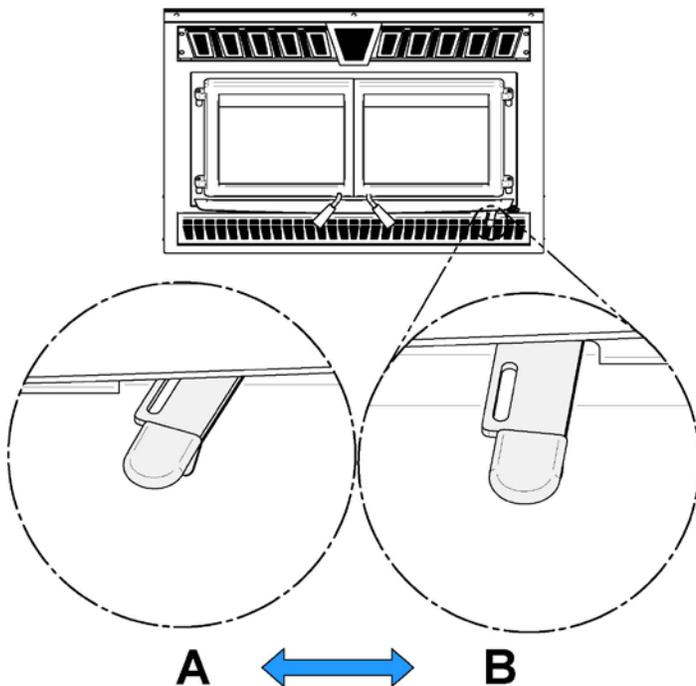
**Position A:** In this position, air supply is fully open. You should be using this position for :
