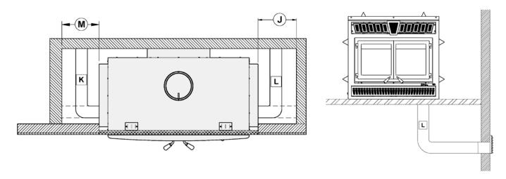
Refer to the building code or the local code for regulations concerning the need to install finishing material inside the chase around the fireplace.
