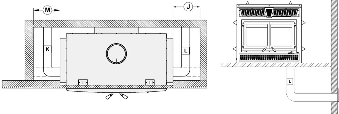
Refer to the building code or the local code for regulations concerning the need to install finishing material inside the chase around the fireplace.
