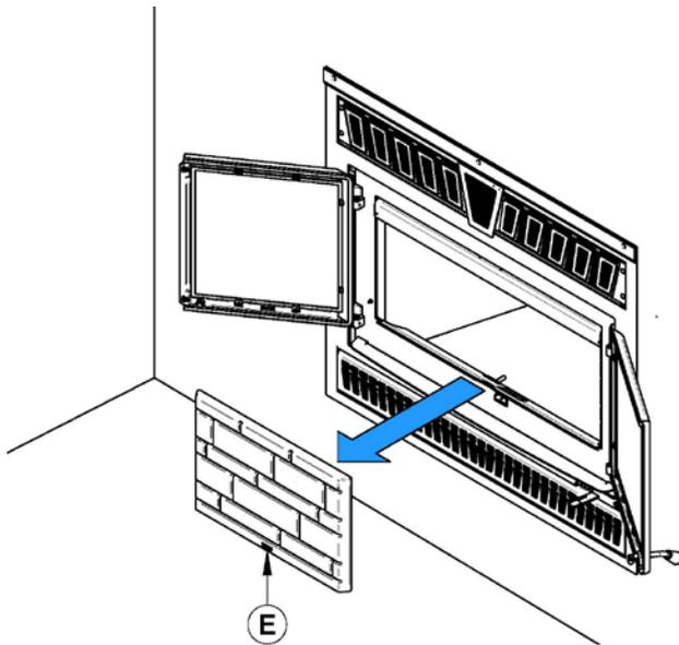
To install new refractory slabs, follow the above steps in reverse.
