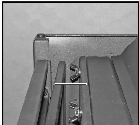
Figure 59: Proper orientation of screen mesh.
