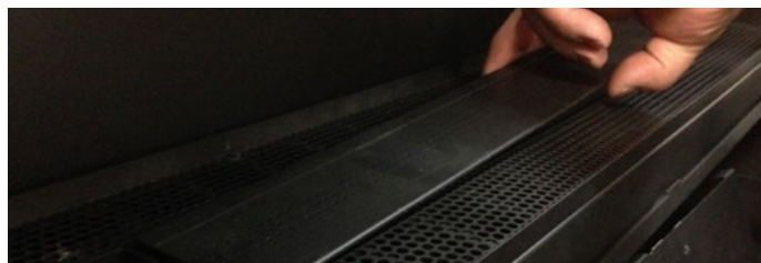
Figure 13.b Loosening the venturi
