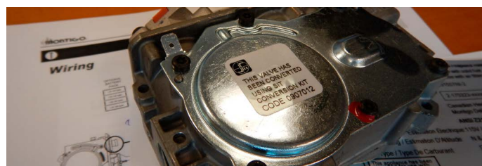
Figure 13.k Conversion label on valve
