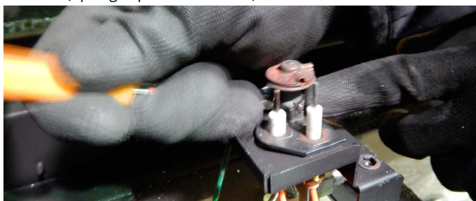
Figure 13.d Removing the spring clip
