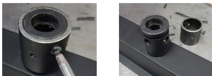
Figure 13.c Removing the orifice
