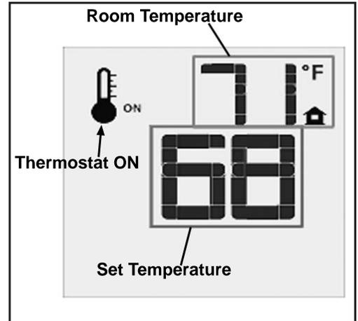
Figure 8: Thermostat Function
