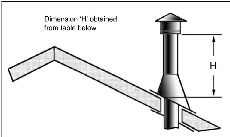
**Figure 74: Height of Vertical Termination;**
