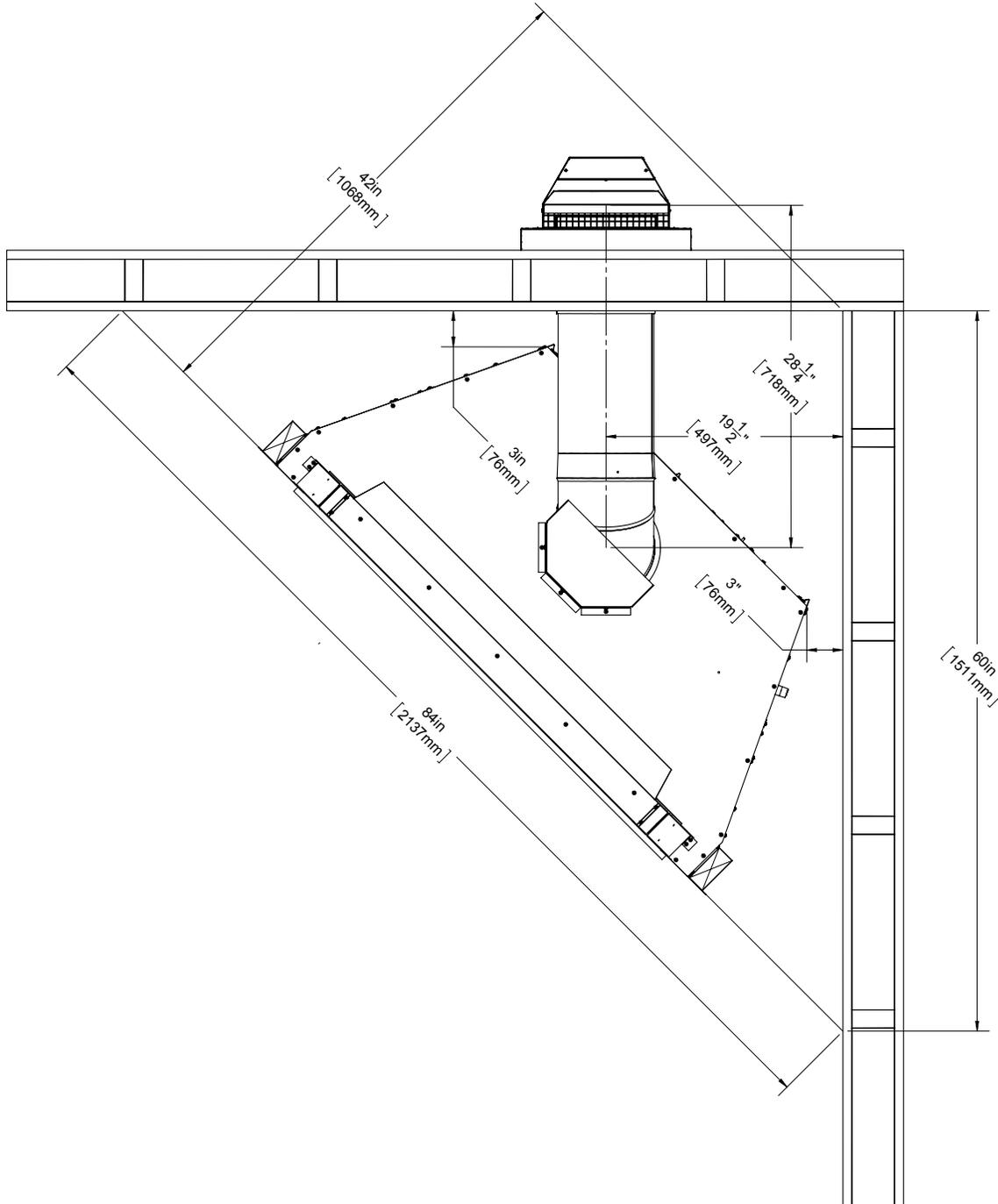
Figure 59. Corner Installation
