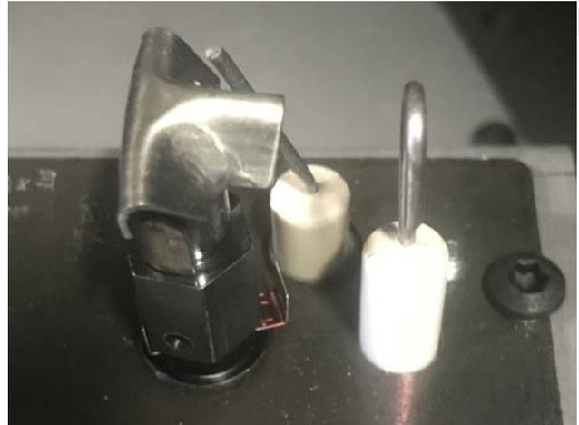
Figure 32: Correct Pilot Position
