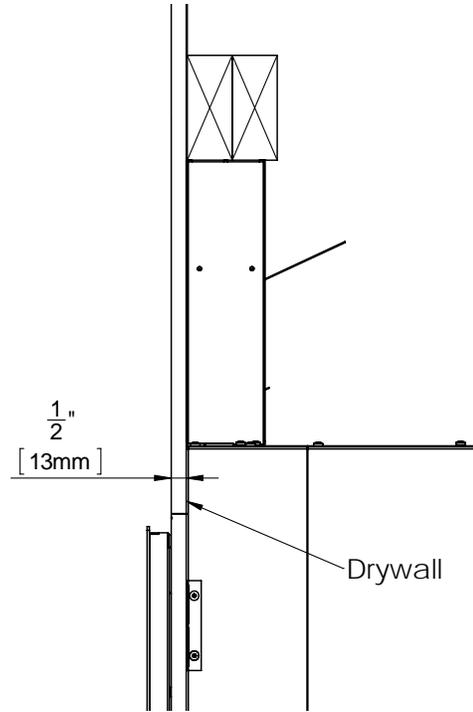
**Standard Extended Install:** Using the supplied long finishing edge, **non-combustible** material may be layered on top of the supplied Non-combustible board. Supplied board not needed for thick **non-combustible** finishes like rock.
