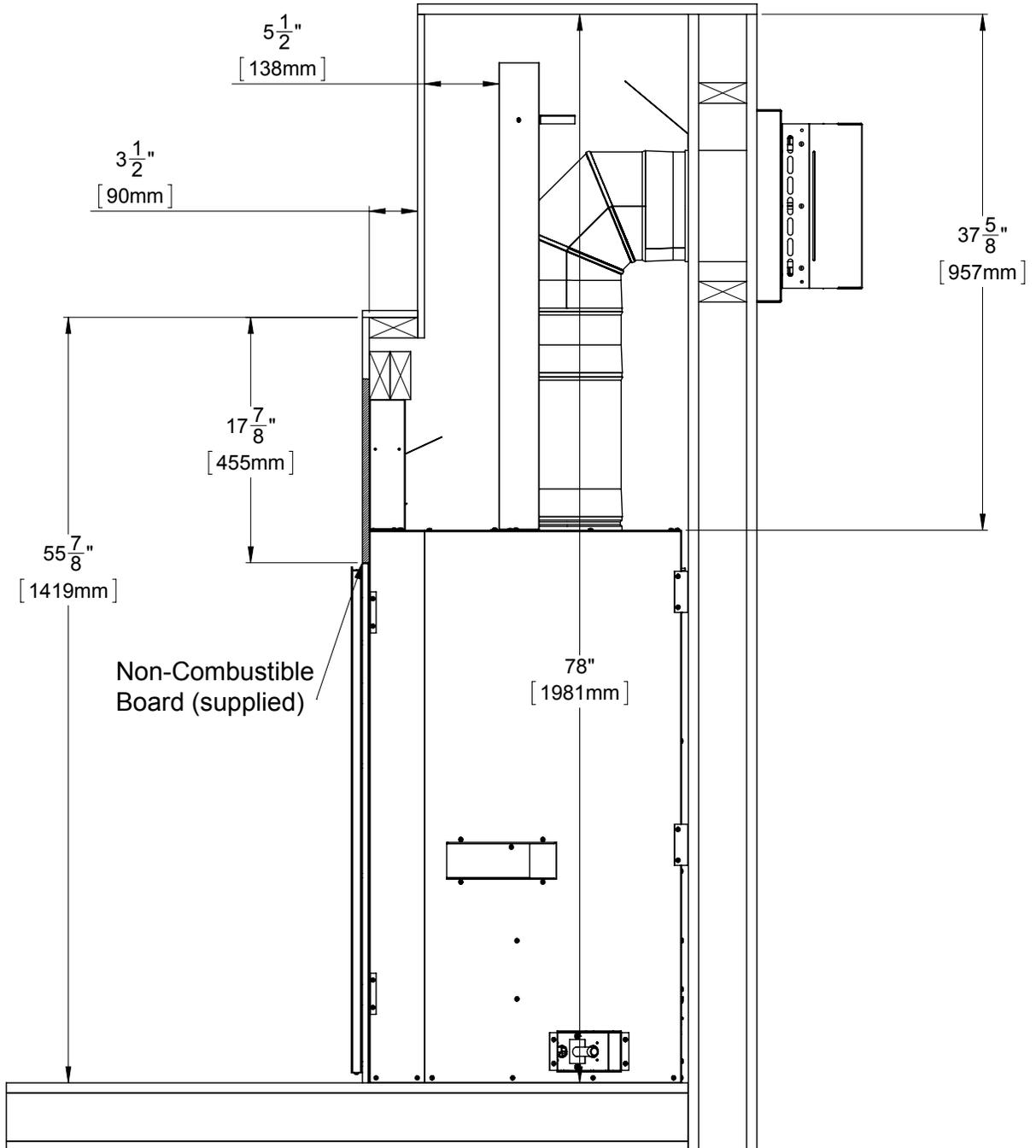
Figure 58: Recess Installation
