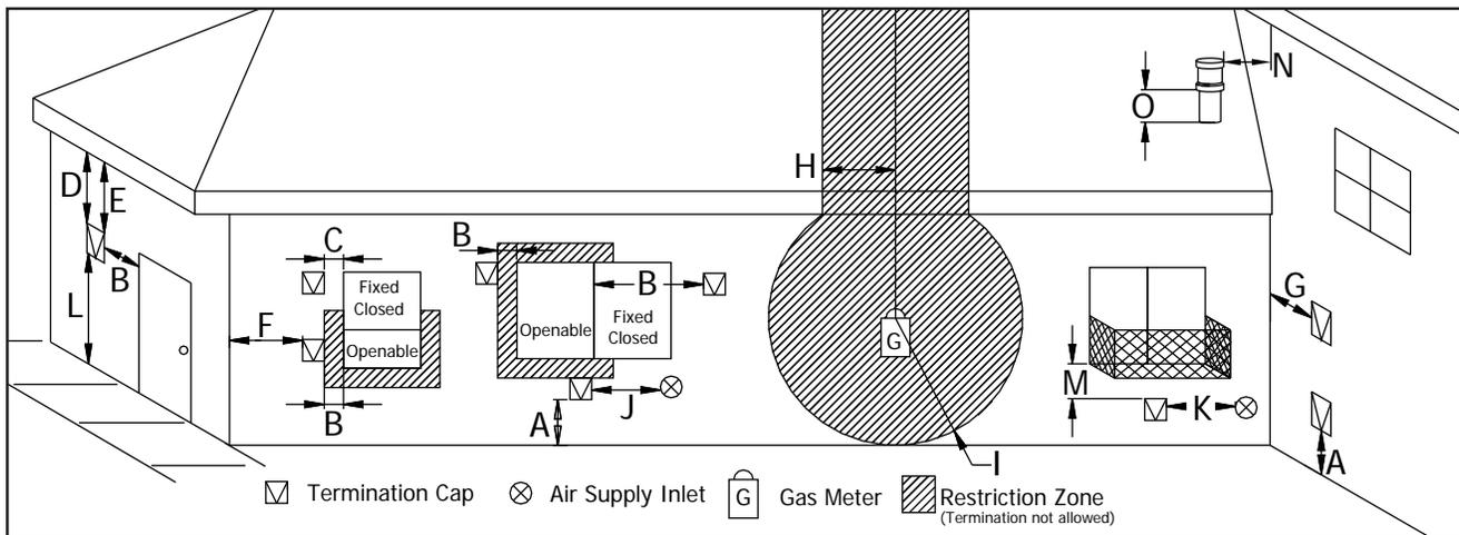
Figure 66. Vent Termination Restrictions, refer to Table 3
