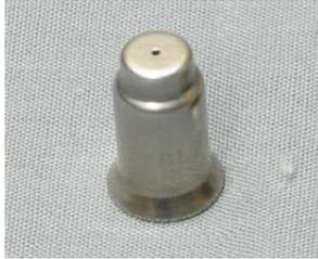
Figure 31: Pilot Orifice
