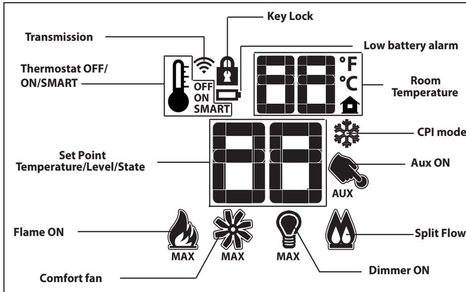
Figure 4: Proflame 2 Transmitter LCD Screen.
