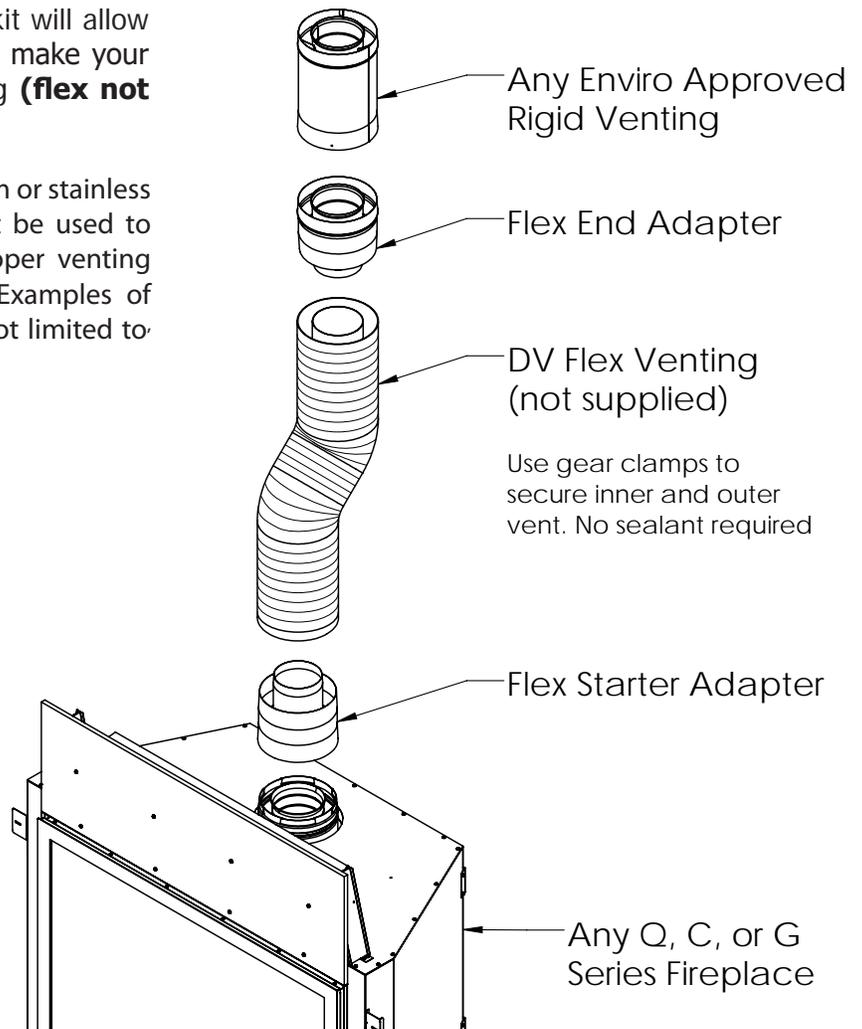
Figure 62. Flex Adapter Kit Install
