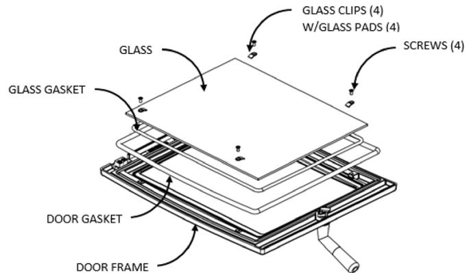
**Figure 20 : Front Door assembly**
