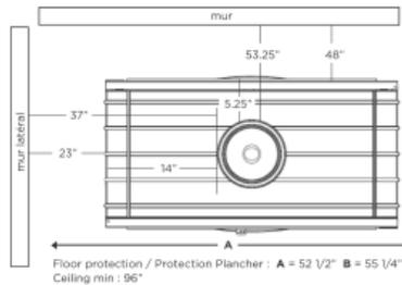
Floor protection / Protection Plancher : A = 52 1/2" B = 55 1/4"
