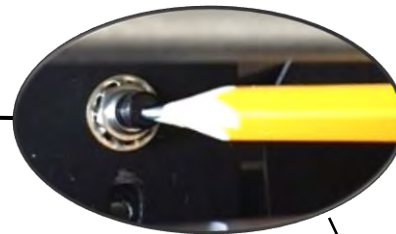
REMOTE PAIRING BUTTON (SW1 SWITCH)
