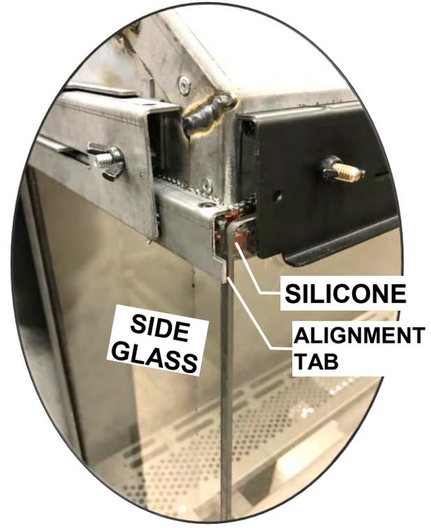
**⚠ IMPORTANT:** Each corner must have a dab of high-temp silicone placed between the ball of the gasket and the corner glass. This will fully seal the firebox corners.
