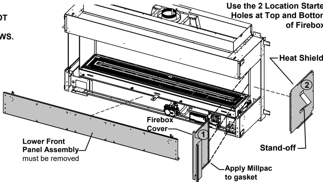
Use [Qty 7] DT Screws to attach Back, Top, and Bottom of Heat Shield
