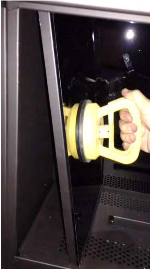
**STEP TWO:** Lift panel in order to place slot in End Panel over Flange on False Bottom.
