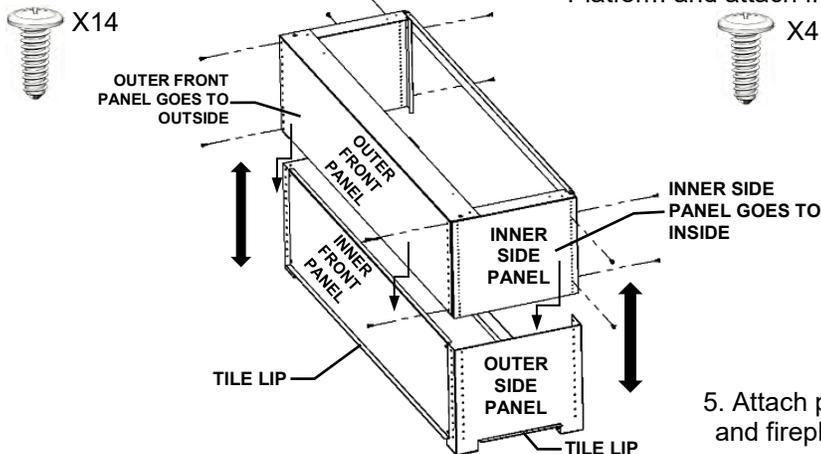
4. Hook back of fireplace into back of Platform and attach front with screws.
