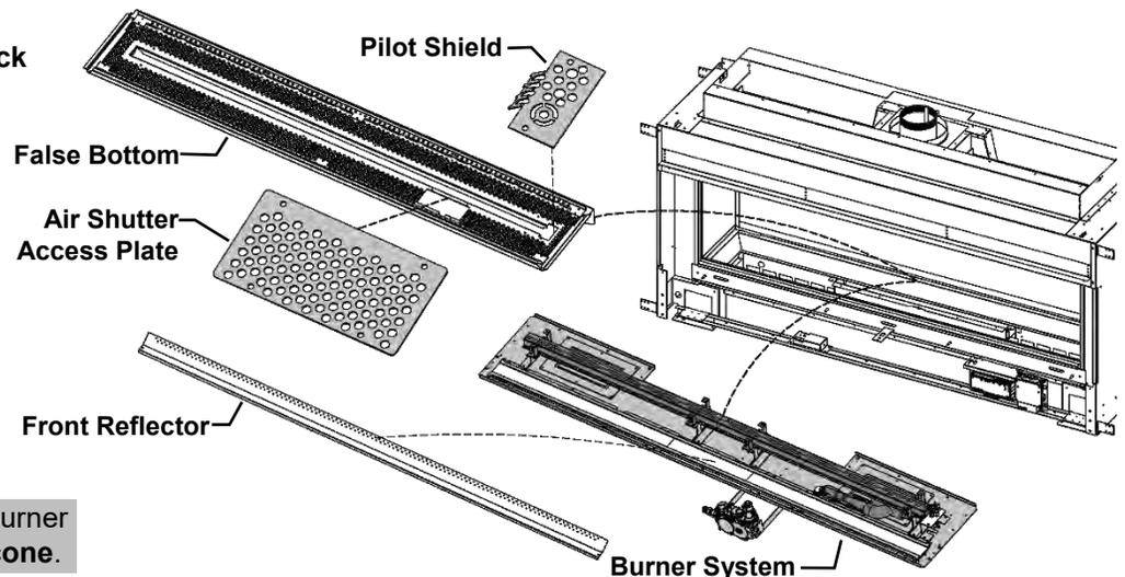
**NOTE:** Pilot connections through Burner Pan must be sealed with **Red Silicone**.
