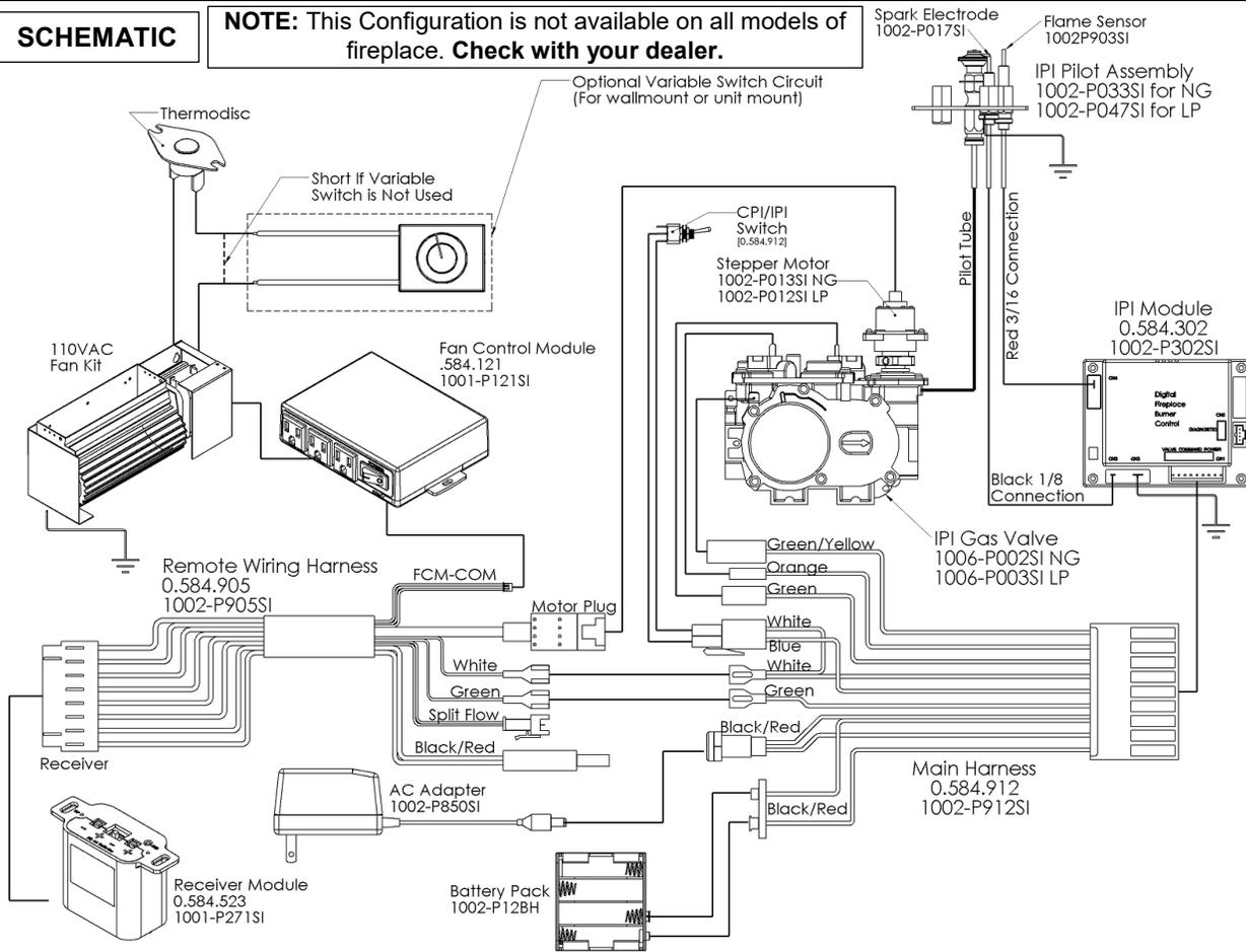
Note: If remote Control is used the battery Pack 1002-P12BH does not need to be used.
