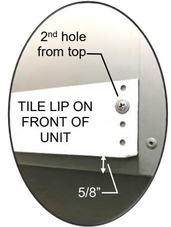
**ASSEMBLY:** Attach Side Fillers and Bottom Filler to Surround Frame with [Qty] 11 screws.
