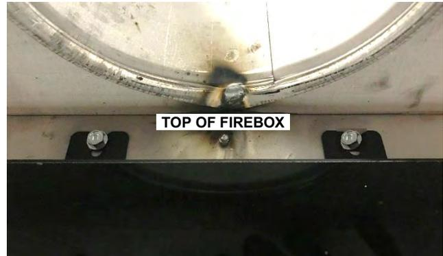
**STEP FIVE:** Reinstall Media Fence as shown, with one row of slots exposed.
