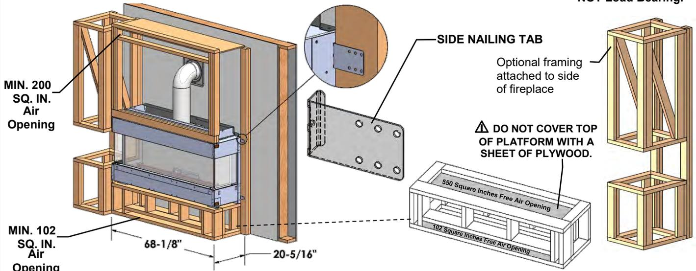
**OPTION B: Framing Attached to Top of Fireplace-** For cantilevered chase.
