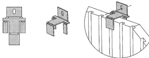
**STEP FIVE: Install Side Liners.** Reinstall End Clips with DT Screws.
