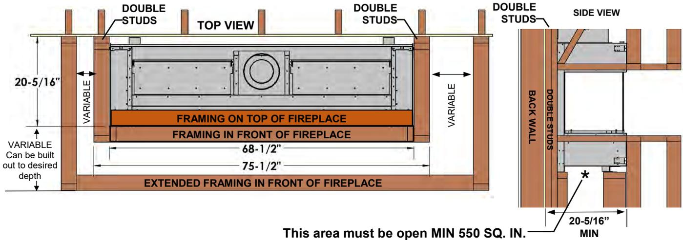
**OPTION B: Framing Attached to Top of Fireplace-** For cantilevered chase. Framing must be self-supporting.
