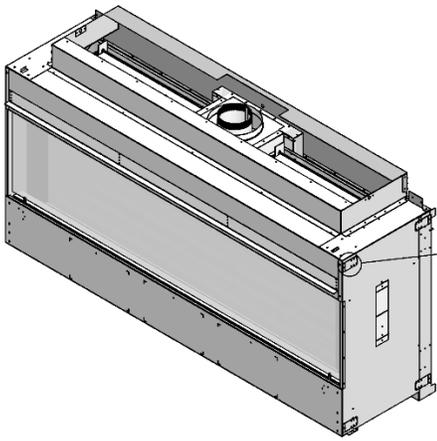
[Qty] 4 Nailing Tabs are located on each side of the front frame.
