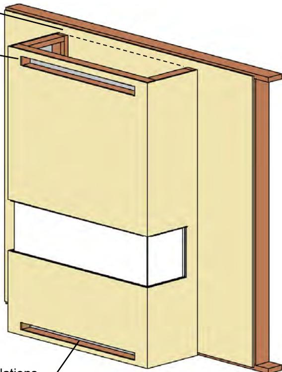
Lower Vent Slot (MIN 102 Sq. In.) is REQUIRED for ALL Installations.
