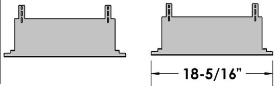
**NOTE:** Install before applying the finishing materials. Install Tile Lip (supplied with fireplace) using second hole from top, as shown. This will provide the required 5/8" clearance above opening.
