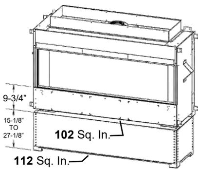
The Adjustable Vented Platform is an optional installation base. Height is variable from approximately 15-1/8" to 27-1/8". Venting slots are provided at the bottom and between the fireplace and the platform.
