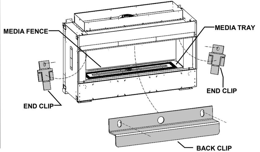
**STEP TWO: Remove Media Fence from Media Tray with [Qty 3] Lower Liner Clips Attached.**
