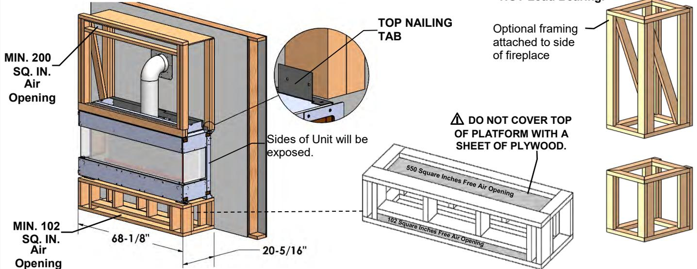
**OPTION C: Framing Attached to Back of Fireplace-** For cantilevered chase.
