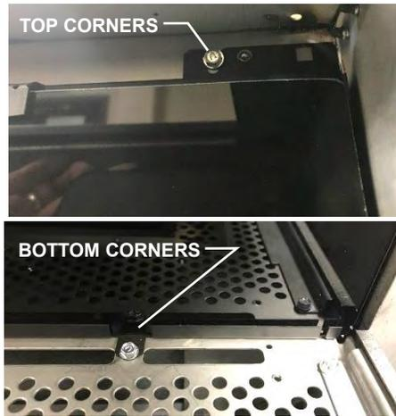
**STEP FOUR:** Install remaining Liner in Center Position in firebox. Attach with 2 DT Screws on top and 2 at bottom.
