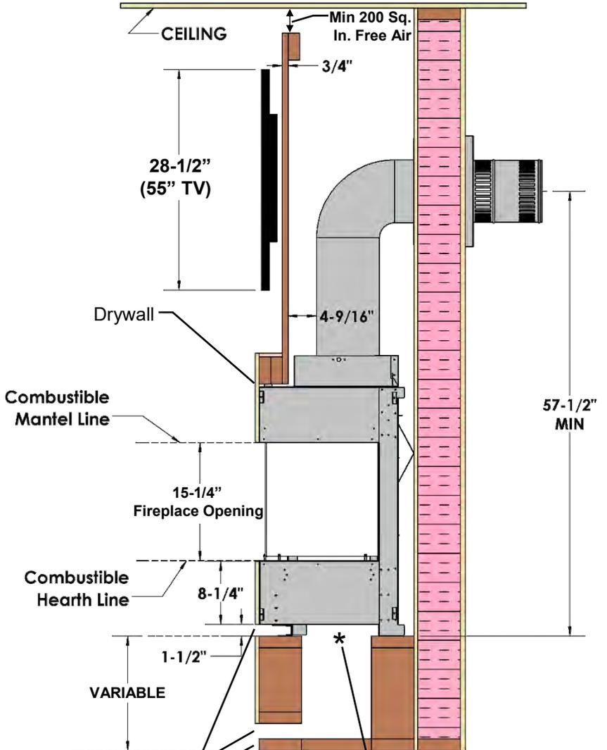
Bottom Air Opening Options – Min 102 sq. in. Opening must not be blocked by floor covering
