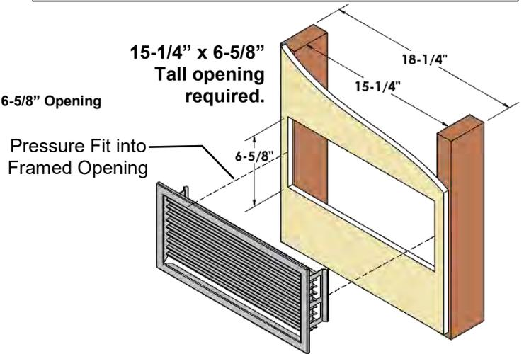
Can be used at Top and/or Bottom of Chase. VL60EGS Grills must be on **Left and Right Side** of chase if used at either location.
