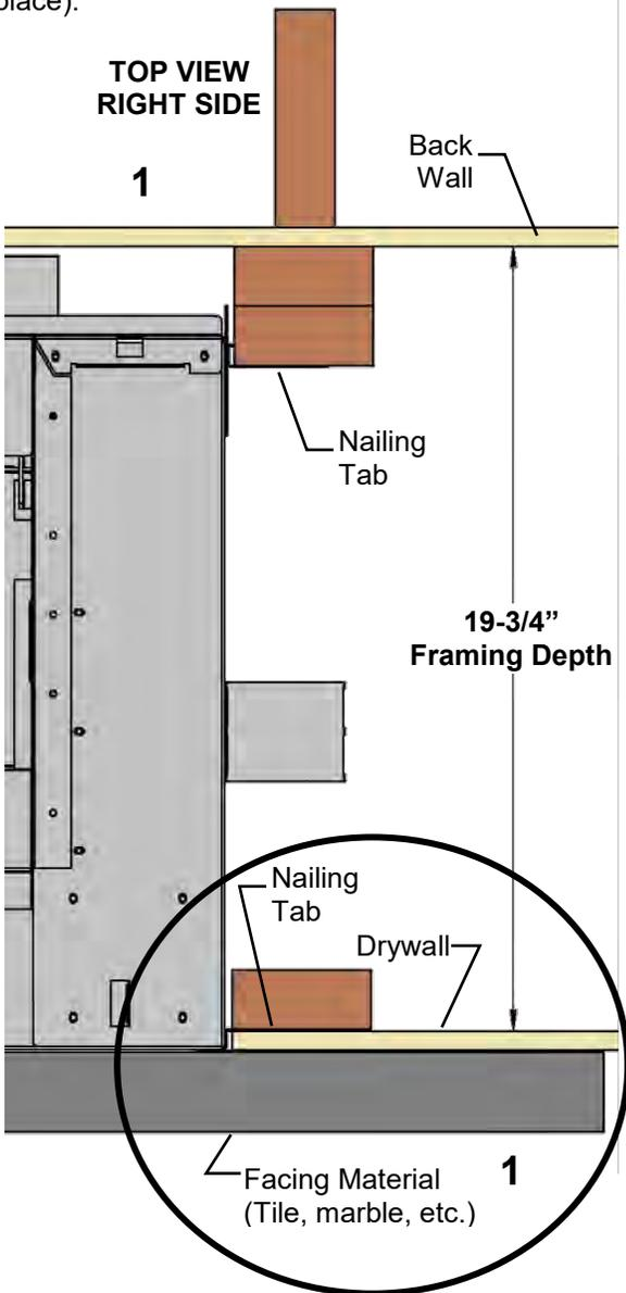
**Framing Flush with Face of Fireplace** –Finished wall surface will continue up to fireplace opening.
