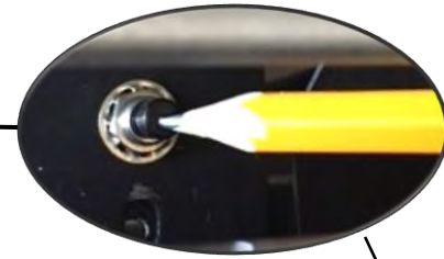
REMOTE PAIRING BUTTON (SW1 SWITCH)
