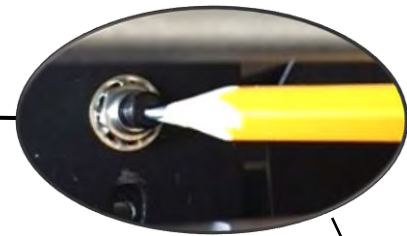
REMOTE PAIRING BUTTON (SW1 SWITCH)
