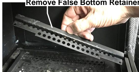
E Remove False Bottom Retainer
