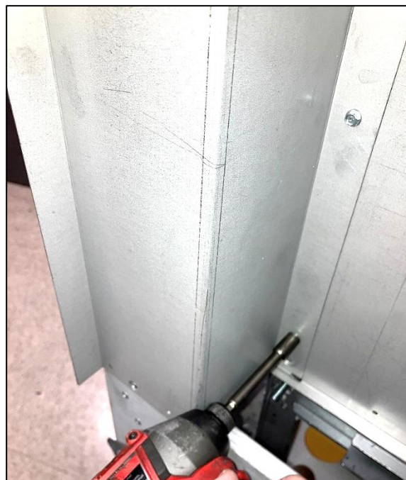
Attach Front Side Cover with DT Screws
