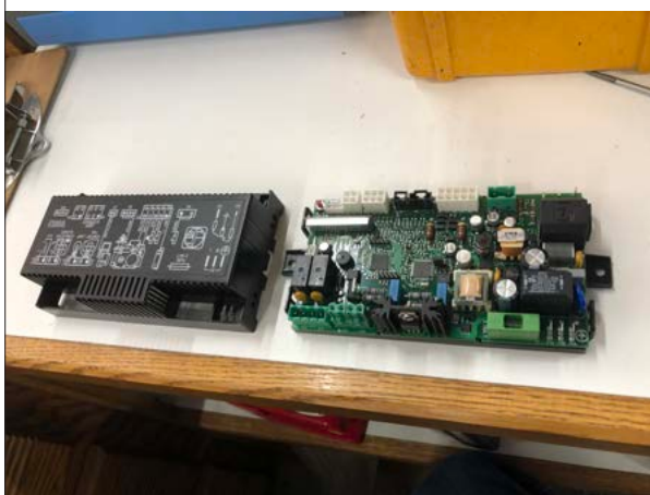
Figure 4.1, Remove Control Board Cover
