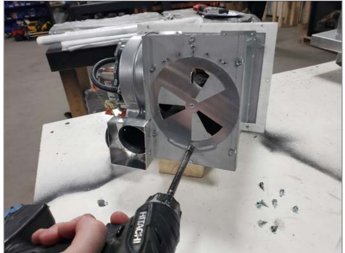
Figure 2.5, Loosen Locking Screw
