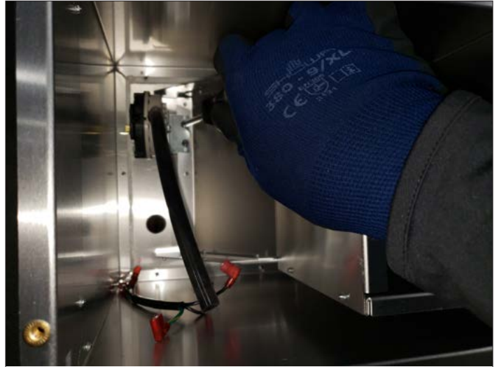
Figure 5.8, Screws Securing Vacuum Switch Bracket
