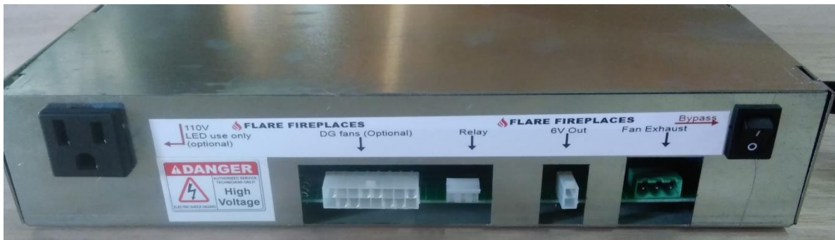
Optional control module for double glass units.
