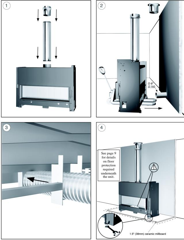
Take necessary precautions to avoid ceramic board from crushing under weight of fireplace.
